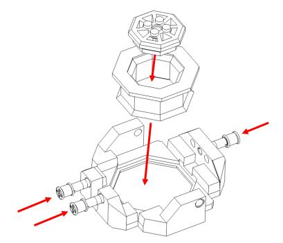
Assemble as shown. Add the three included technic push pins as shown
