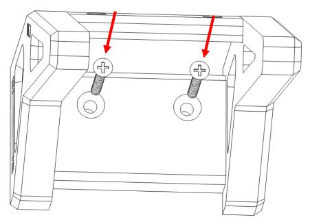
Do not over tighten the screws (do not use a drill to tighten)
