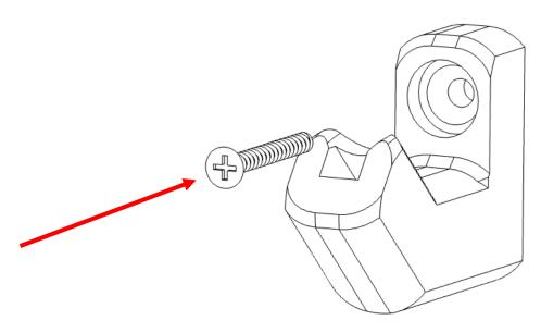
Do not over tighten the screws (do not use a drill to tighten)
