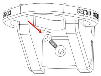
Do not install the screw with a drill driver. Use a screwdriver and do not over tighten.
