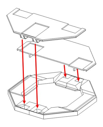
You can orientate the set to face angled either left or right by fitting the frame in at a 45 degree offset.
