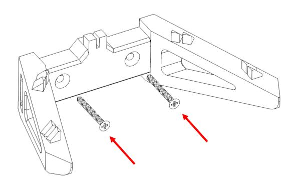
Use the provided wall fixings to secure to the wall. Do not over tighten the screws (use a screwdriver only).
