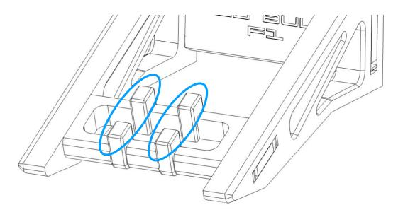
These tabs insert into the frame of the Lego set, Line up the tabs with the corresponding locations on the Lego set.
