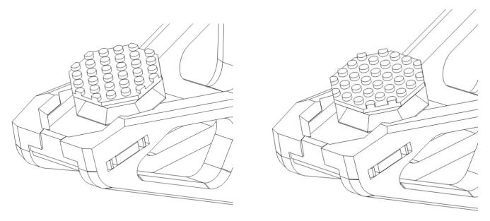
Mount the adaptor piece under the set at the centre of balance.
