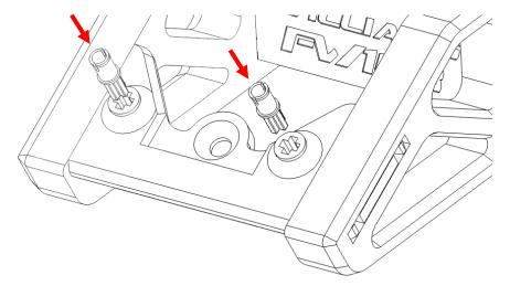
Use the two blue pins from the original Lego set display mount
