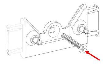
Use just the front plate as a flush wall mount. You can orient the plate in any direction to suit your preferred display orientation
