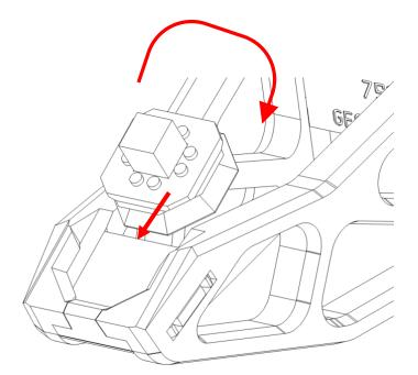
Mount the adaptor piece under the set at the centre of balance.
