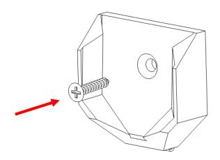
Adaptor piece can be rotated 45 degrees and slide into place in 8 directions.
