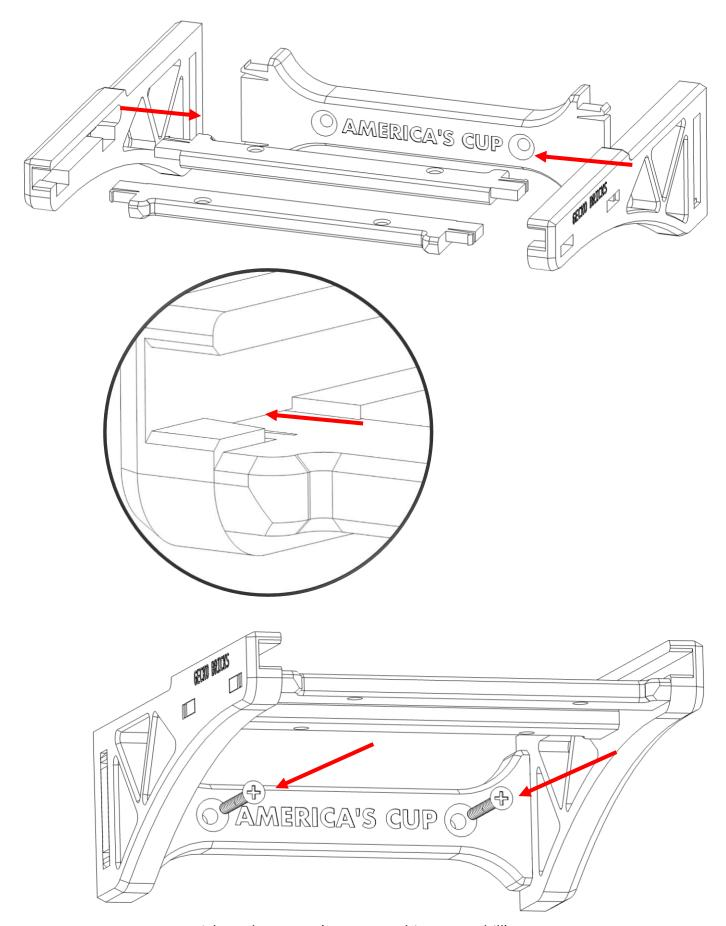
Do not over tighten the screws (use a screwdriver not a drill).
