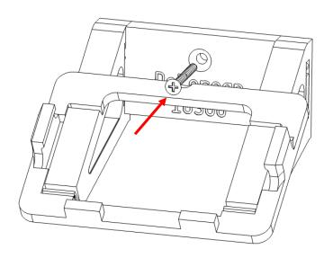
Use the included screw and wall plug to secure the wall mount. Do not overtighten the screw.
