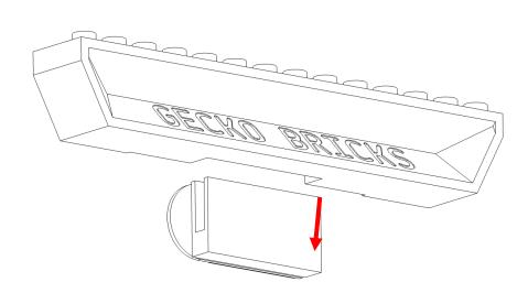
Attach the Minifigure mount lug to the wall first
