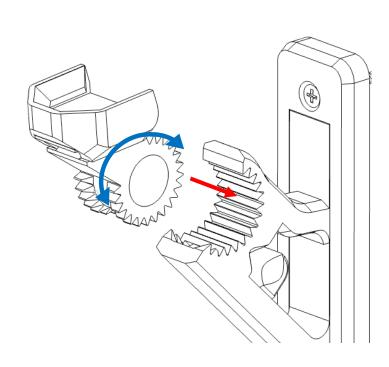
You may adjust the angle of the set by repositioning the angled adaptor
