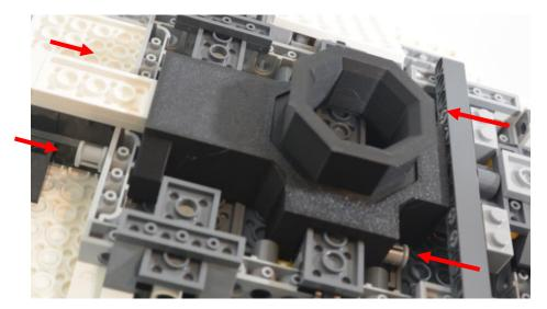
With the adaptor assembly seated in the Lego set push the 4 included Techinc pins to secure in place
