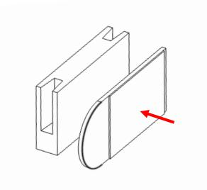
Use the 3M command strip to adhere the cleat to the wall. Press firmly to fully adhere the command strip.
