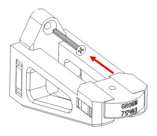
Do not over tighten the wall screw
