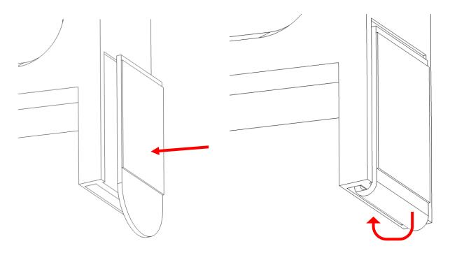
Use the included 3M command strip to prevent the mount from rotating around the fixing.
