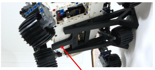
Locate the mounting ledge into the frame of the vehicle. Can be mounted facing left or right.
