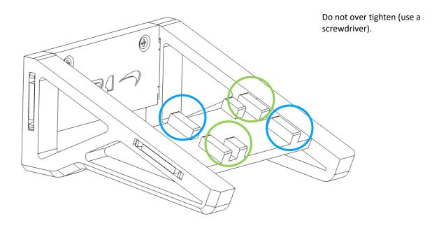
These tabs insert into the frame of the Lego set, Line up the tabs with the corresponding locations on the Lego set.
