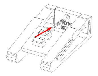
Install screw into the wall stretcher. Do not over tighten (use a screwdriver).
