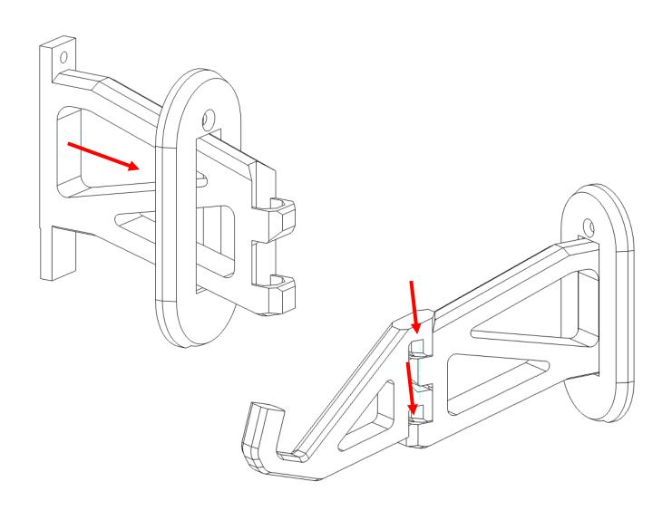
Fit the outer arm at 45 degrees Left or right
