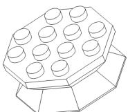
Mount the adaptor piece under the set at the centre of balance.
