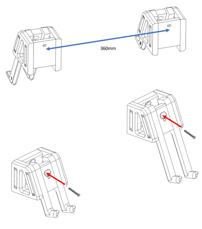
Adjustment left and right for any misalignment in the next step
