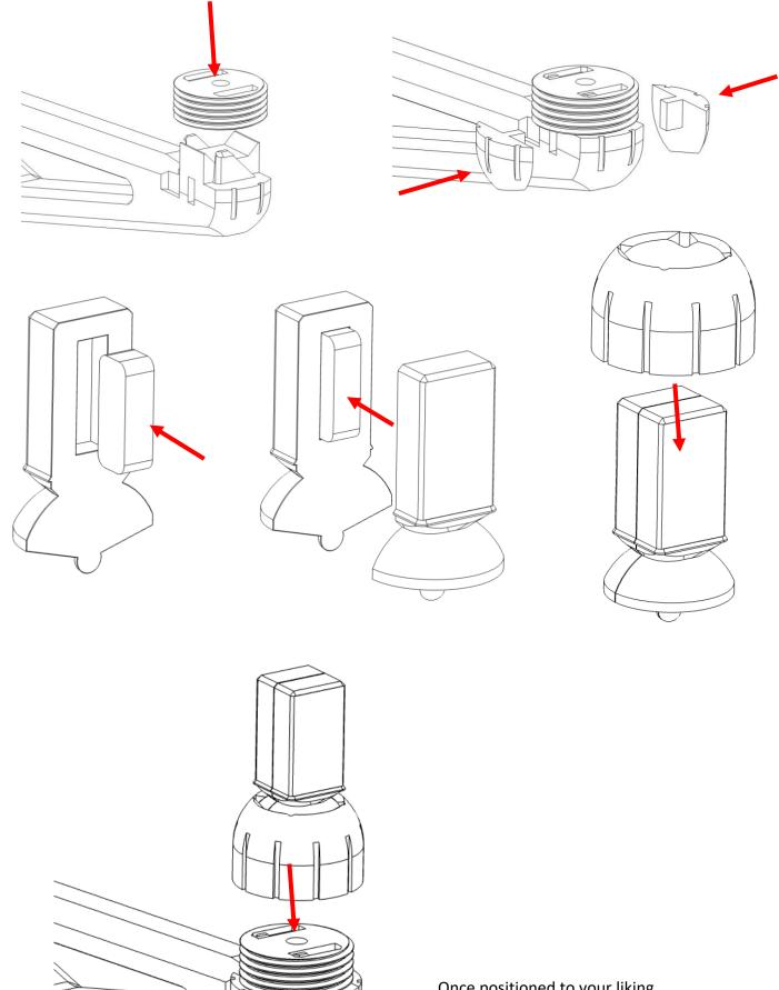
Once positioned to your liking, you can gently tighten the screw cap to secure the ball joint in place.
