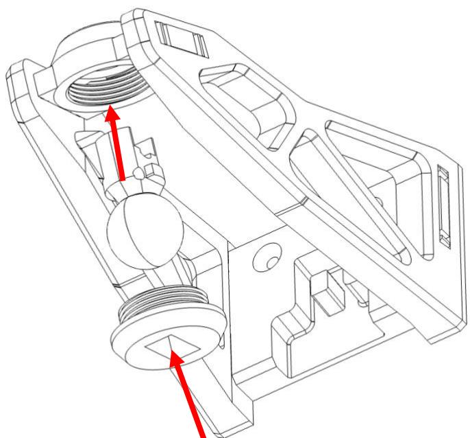
Feed the ball joint through the lower stretcher and screw the ball joint cap on to secure it in place.
